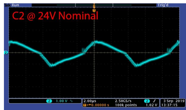
Fig. 18 Voltage waveform of flying capacitor C_2 at full load(using capacitors as designed in Tab. 4)
