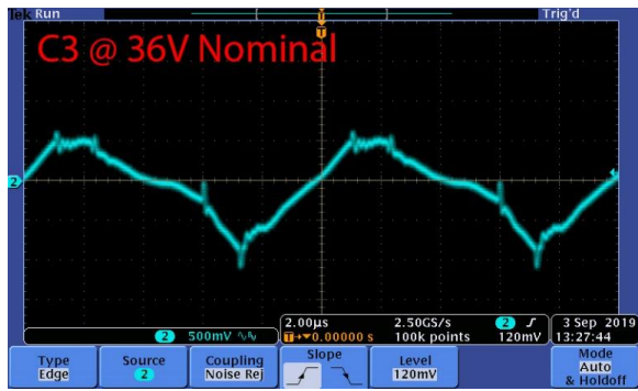
Fig. 19 Voltage waveform of flying capacitor C_3 at full load (using capacitors as designed in Tab. 4)
