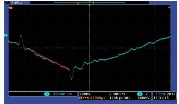
Fig. 10 Magnified voltage waveform of C_3 (centered around the instance where it is carrying full load current)
